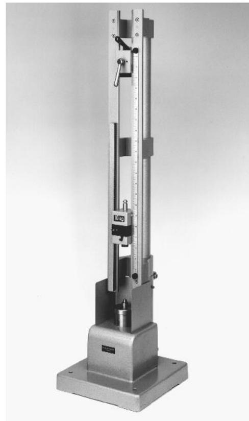
faces  $r_a=0.08 \mu\text{m}$ )④, a hollow steel collar (Ø16 mm; height: 13mm; polished bore of  $10_{+0,010}^{+0,005}$ ) ⑤ and a centring ring (13) for fixation. The assembly is placed onto a small anvil 26x26mm (12).
